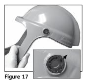
To aid assembly for installing the outer door on the HMX helmet, remove the shroud retainer and suspension from the helmet shell.
