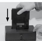
Place battery upside down into the charging port of the battery charger. (Figure. 2)
