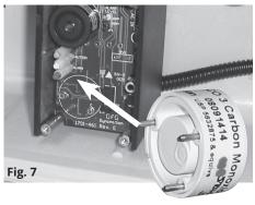
Align pins and gently push the new sensor into the sockets (Figure 7).
