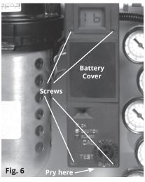
The sensor is easily accessible by removing the front of the housing from the COM5 or COM10 monitor.
