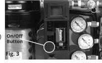
The knob must be in RUN position for active monitoring of CO in the air supply.
