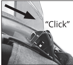
5) Align the visor over each retainer, matching the notch with the button and push until you hear a click.
