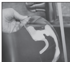
4) Clean visor with mild soap, rinse thoroughly with clean water, and dry with a soft cloth
