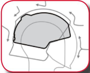
The layout of the platform, outer shell and visor encloses the inner compartment hermetically against all risks. No comparable helmet offers a similar protection against heat, flames, sparks and fluids.
